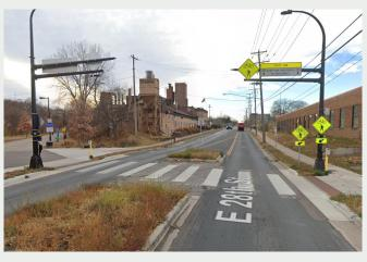
Pedestrian hybrid beacon - a flashing yellow and flashing/solid red signal that increases motorist stopping rates. Credit: Red Wing, MN Google
