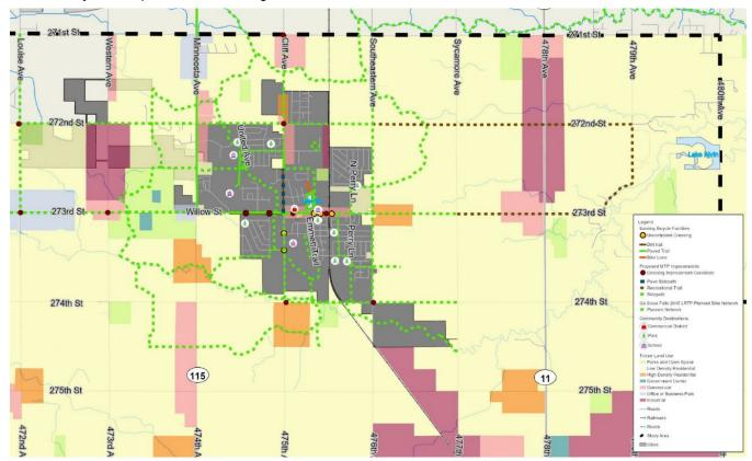
**Figure B.4:** Proposed bicycle and pedestrian improvements include crossing improvement candidates (brown circles), paved sidepaths (blue dotted lines), recreational trails (brown dotted lines), and sidepaths or the planned bike network from the Sioux Falls Long Range Transportation Plan (green dotted lines).
