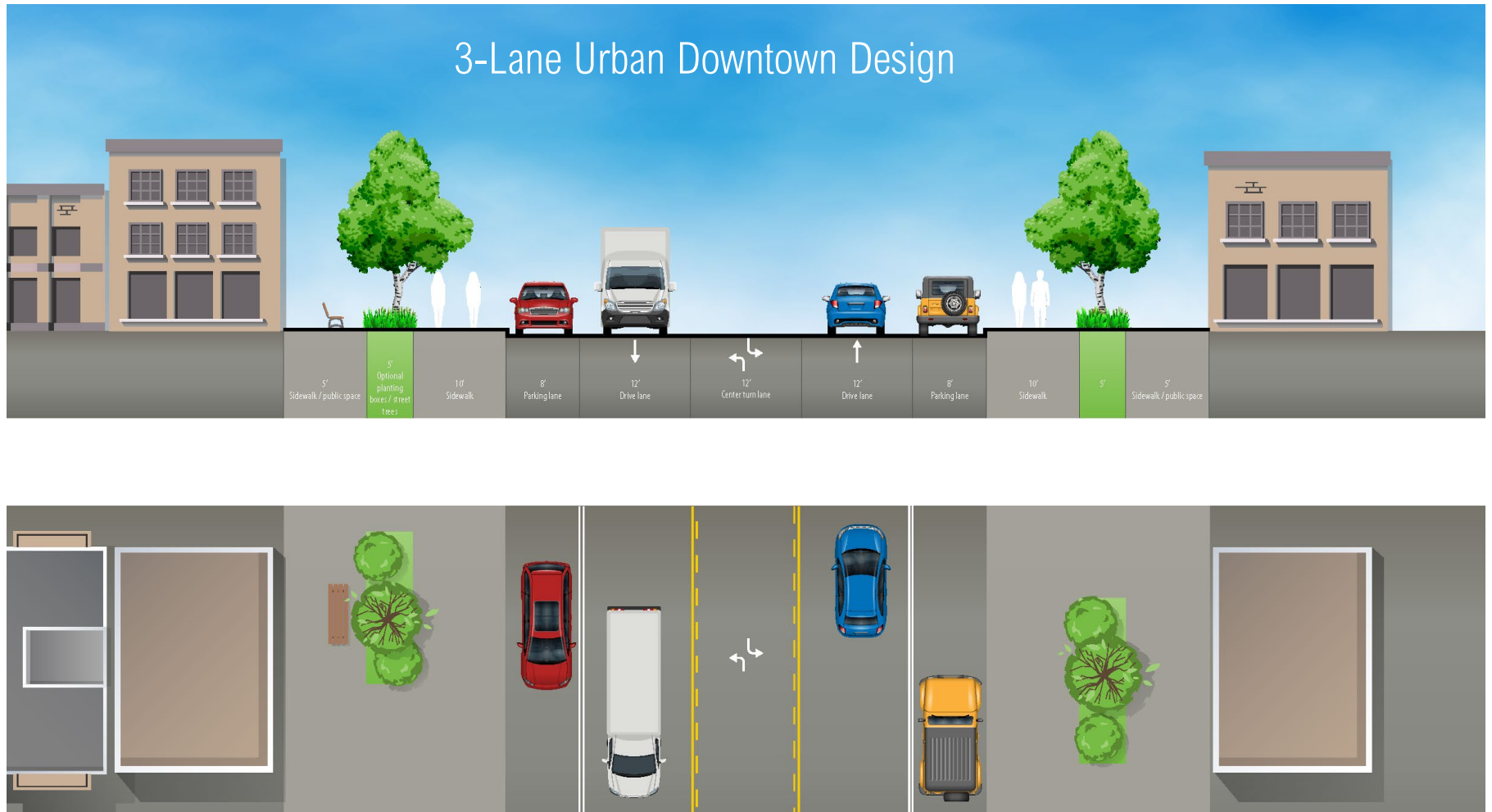
Figure 25: 3-Lane Urban Downtown Cross Section (100' Right-of-Way)
