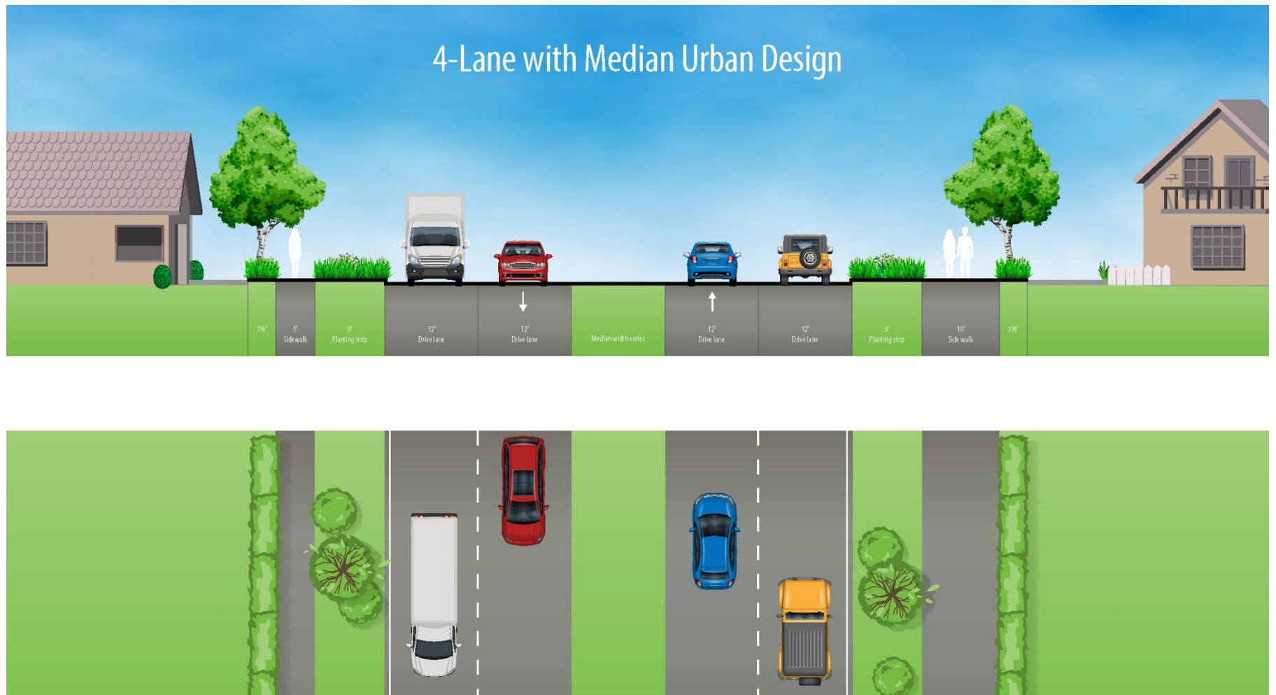
Figure 24: 4-Lane Urban Cross Section with Median
