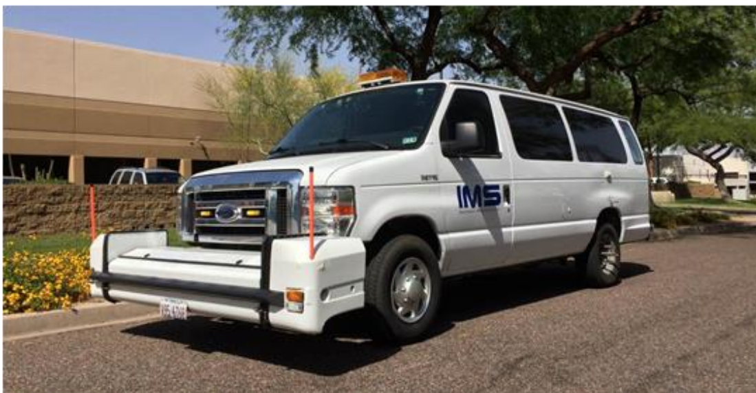
Figure 4 – Laser Road Surface Tester (RST)
