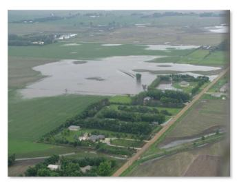
Drawing 10 also highlights natural storage north of 272<sup>nd</sup> Street, adjacent to Harrisburg Homesites Addition. An existing 8" drain tile is the only discharge relief at his location, and results indicate the natural storage area does not overtop 272<sup>nd</sup> Street during the 100-year rainfall event. The picture on the right was taken June 18, 2014 shortly after a significant rainfall event.
