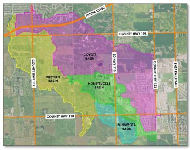
tributary branch of Nine Mile Creek drains Coyote and Honeysuckle basins and reaches as far north as Sioux Falls and convey storm flows through the City of Harrisburg. All runoff from the contributing basins that are included in this analysis discharge into Nine Mile Creek and is eventually conveyed east to the Big Sioux River. Numerous intermittent tributaries extend north and south of Nine Mile Creek, draining the adjacent uplands.
