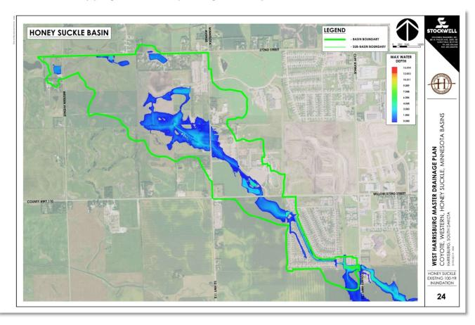
Moving downstream along the main line channel, a site specific storm water detention facility that serves the High School intercepts runoff, just north of Willow Street before crossing through a 6'x3' RCBC without overtopping the roadway. As runoff is conveyed downstream, runoff enters another small detention pond that provides limited storage
